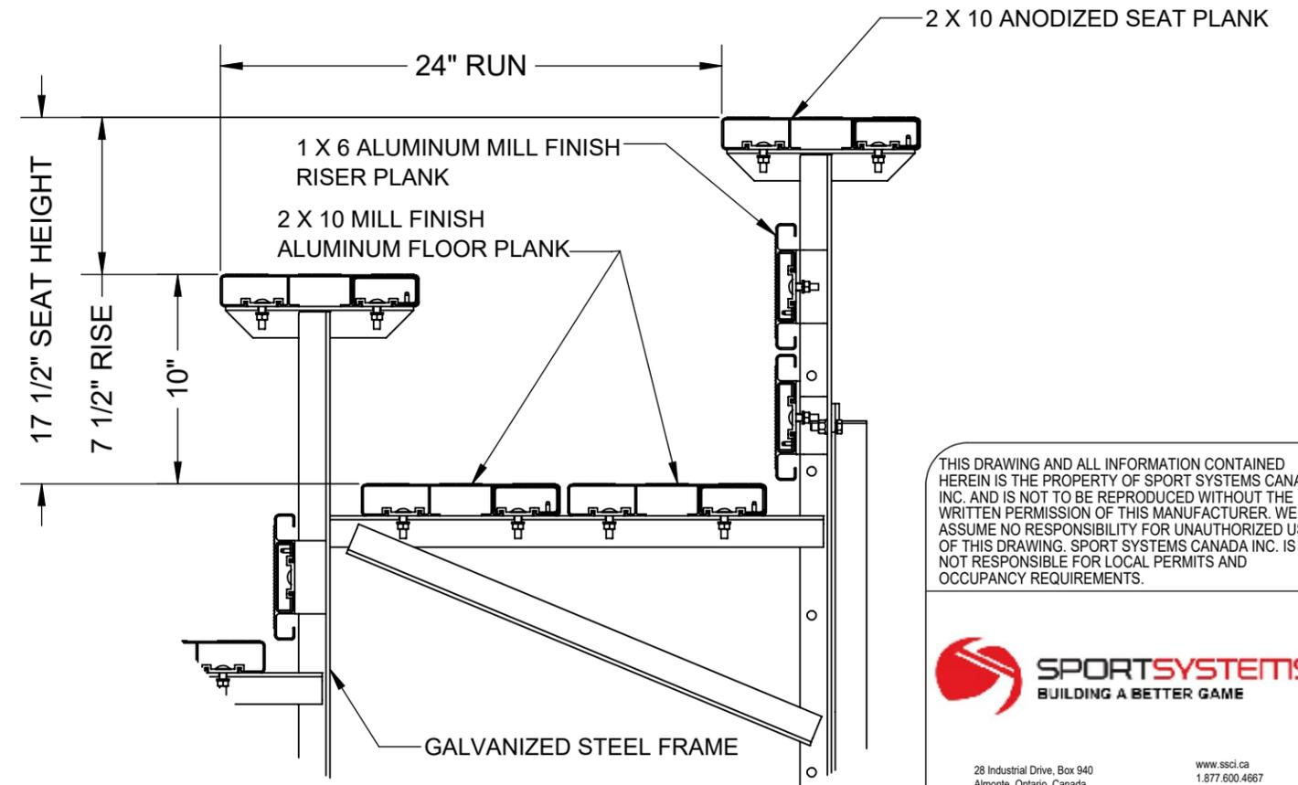
TYPICAL SEAT AND FLOOR BOARD DETAIL
